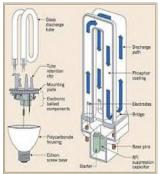
Compact florescent lamps (CFLs) produce light differently than incandescent bulbs. In an incandescent, electric current runs through a wire filament and heats the filament until it starts to glow. In a CFL, an electric current is driven through a tube containing argon and a small amount of mercury vapor. This generates invisible ultraviolet
