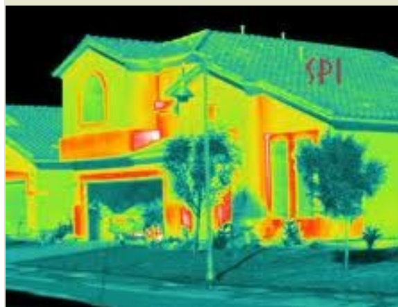
Energy audits will help ensure the energy efficiency of each home, yielding long term savings for residents. The type of audit shown above shows the extent of leaks in the building envelope with the help of infrared cameras.
